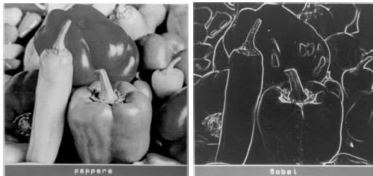
figure: Edge Image using Sobel operator (a) Original image, edge detection using threshold value (b) 110, (c) 90, (d) 70.
