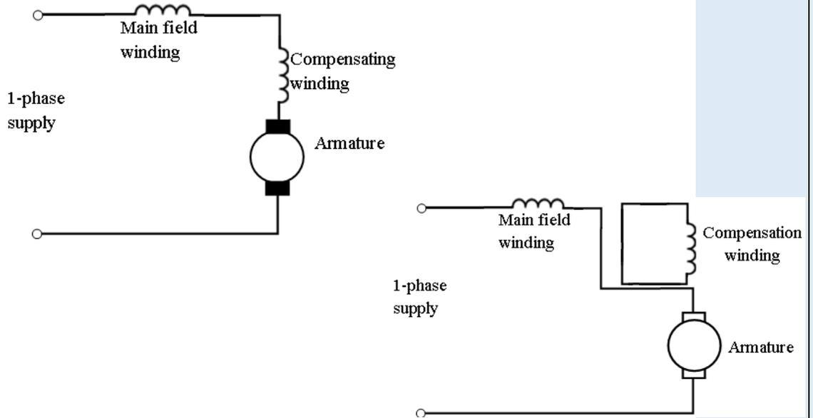
**Like DC series motor. The speed of a universal motor is low at full load and very high at no load. Usually, gears trains are used to get the required speed on required load**
