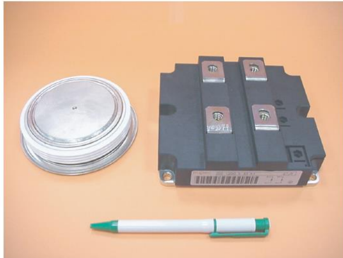
4.5-kV/0.8-kA press-pack and 1.7-kV/1.2-kA module diodes.
