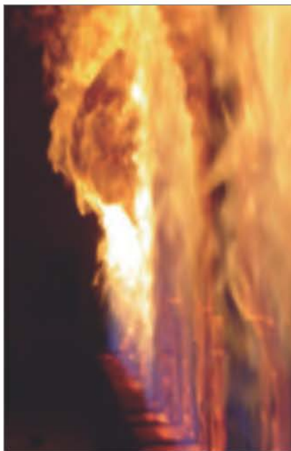
Figure 4a Flooded, fuel rich firebox
