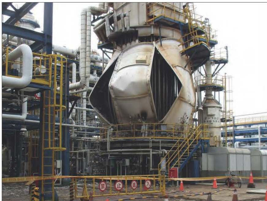
Figure 6 Heater incident resulting from flooding (Courtesy of NOWnews)
