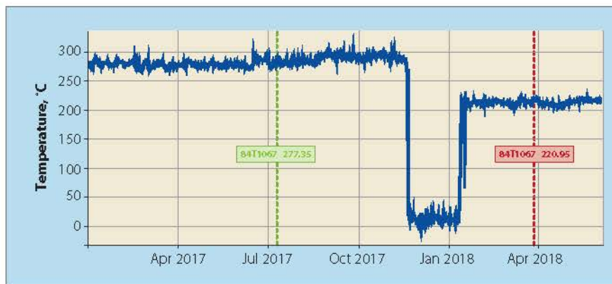
Figure 3 SMR furnace flue gas temperature leaving the stack, before and after cleaning
