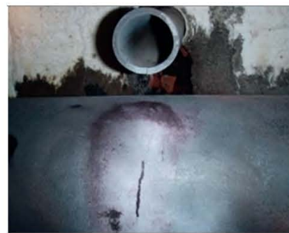
1b Cause found to be snuffing steam condensate dripping on the tube over time
