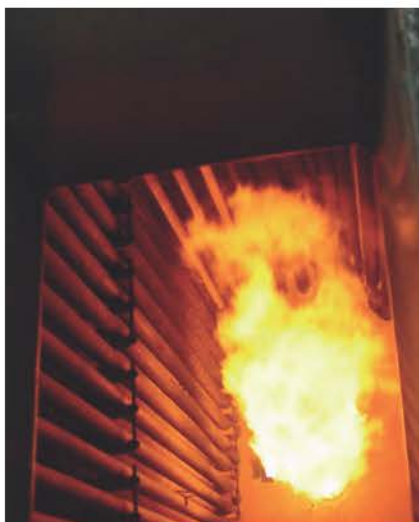
Figure 5 Fuel rich flame impinging on convection section tubes
