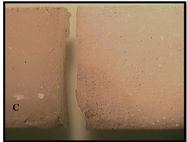
Figure (4.11) :A. show the fail in control sample, B. show the fail in 2% (HA), C. show the fail in 5% (HA).
