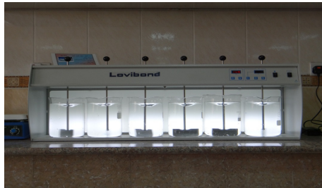
Figure 4 A photograph for the Jar test apparatus used in the study type Lovibond model MT 740.
