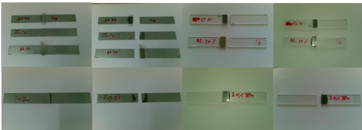
Figure(4) acrylic and galvanized steel specimens before and after the shear test
