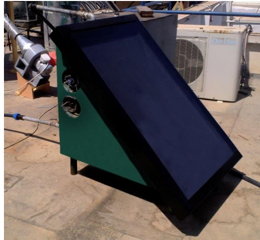
Figure (2) The new integrated solar water heater.
