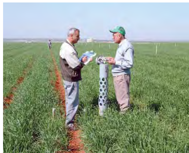
The neutron probe or TDR allows quick measurement of soil water status on research station fields.
