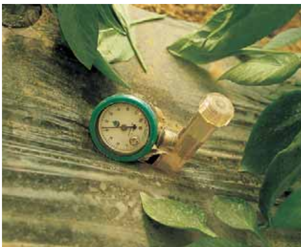
Tensiometers are not suitable for scheduling supplemental irrigation.
