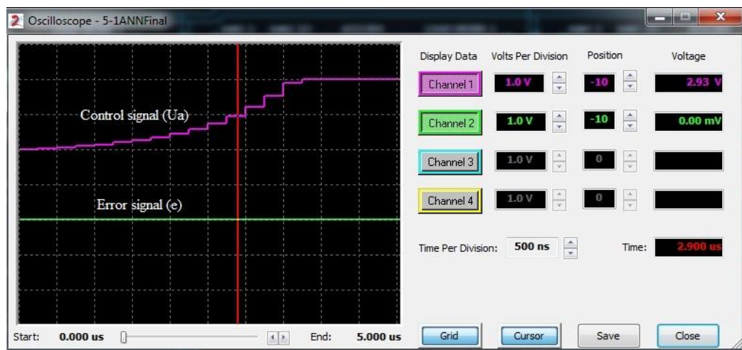
Fig. (17): Control signal ( U_t ) output from seventh FPAA was realized in Anadigm Designer 2 to control the speed of a dc motor
