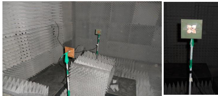
Figure (9): The transmitter and receiver positions in the anechoic chamber
