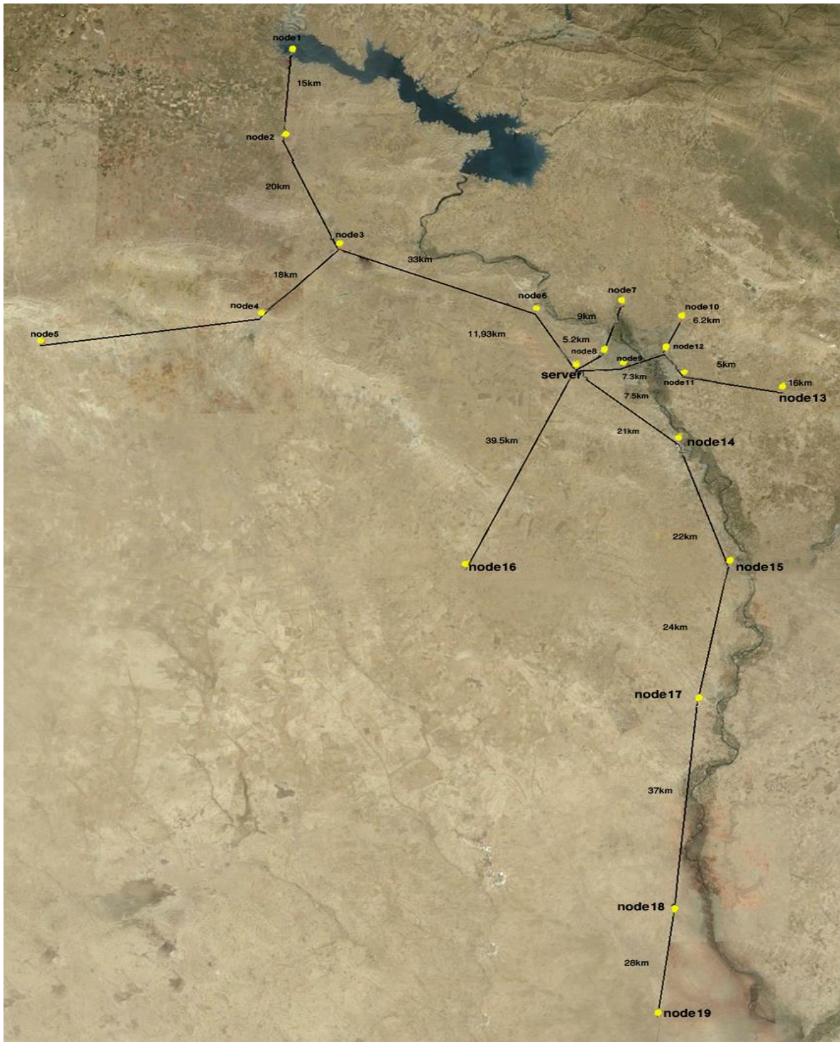
Figure 3. Substations locations on Mosul city map (using Google earth software)
