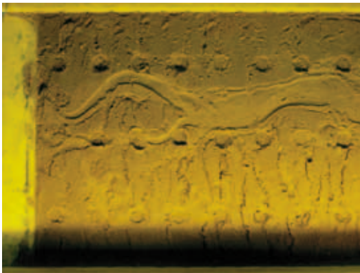
Small-scale piping experiment
