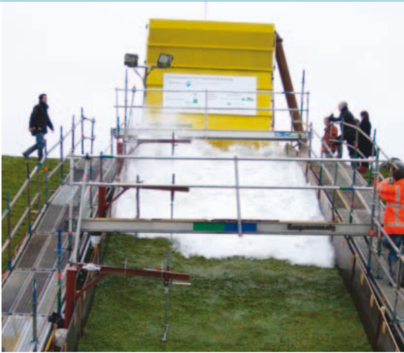
Experiment with the Wave Overtopping Simulator
