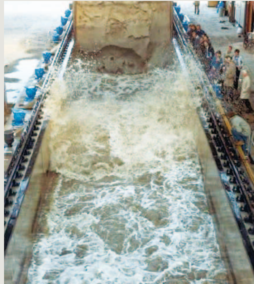
The Delta Flume in action: testing dune strength
