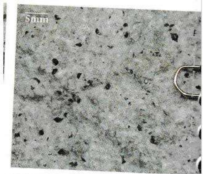
(c) Fine grained (most grains too small to see with the naked eye—less than 0.5 mm across).
