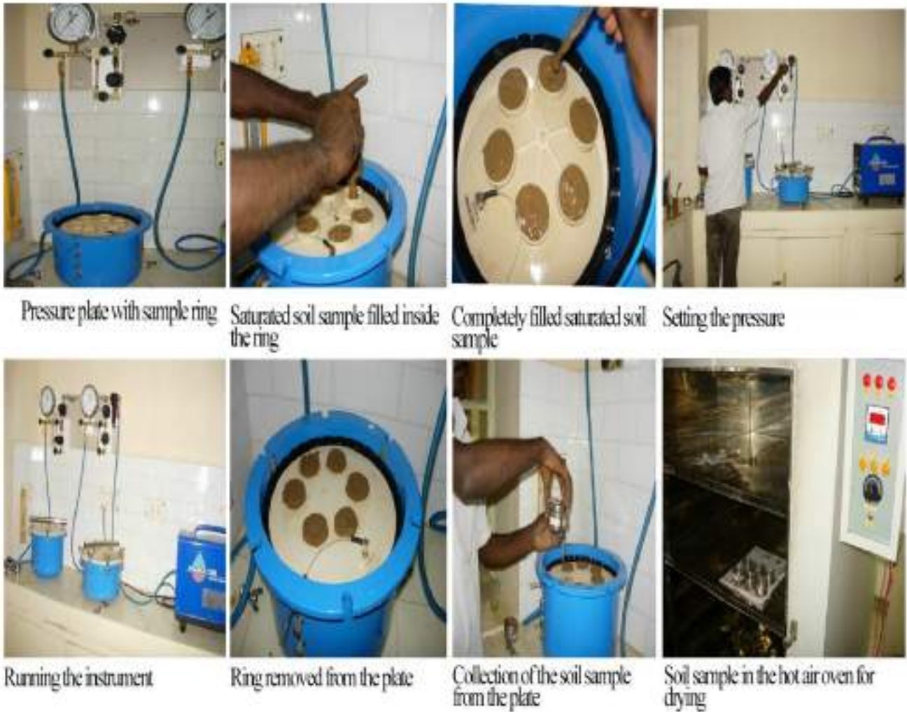
Figure 1 Soil moisture measurement by using Pressure Plate Membrane Apparatus
