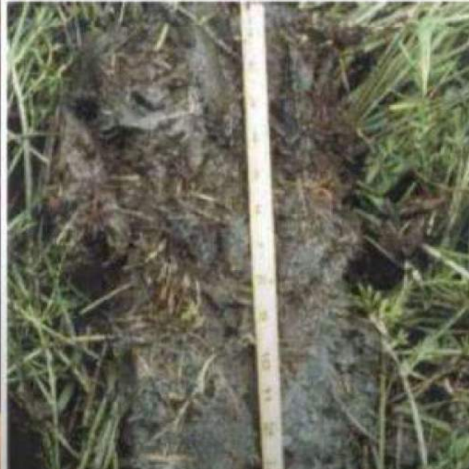
Figure 22. Indicator F2 Loamy Gleyed Matrix. The gleyed matrix starts at the soil surface. Scale is inches.
