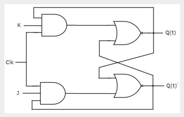
This circuit has two inputs J & K and two outputs Qt & Qt. The operation of JK flip-flop is similar to SR flip-flop. Here, we considered the inputs of SR flip-flop as S = J Qt and R = KQt in order to utilize the modified SR flip-flop for 4 combinations of inputs.
