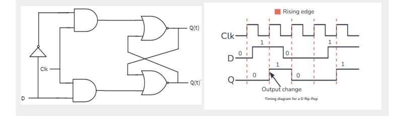
This circuit has single input D and two outputs Qt & Qt. The operation of D flip-flop is similar to D Latch. But, this flip-flop affects the outputs only when positive transition of the clock signal is applied instead of active enable.
