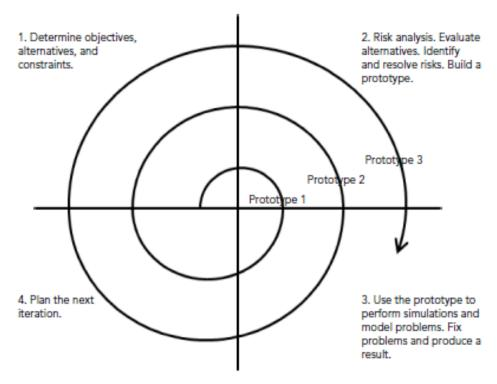
The spiral process uses four phases.
