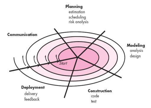
The first circuit around the spiral might result in the development of a product specification; subsequent passes around the spiral might be used to develop a prototype and then progressively more sophisticated versions of
