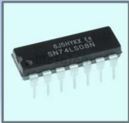
The TTL quad-2 input AND gate (7408)
