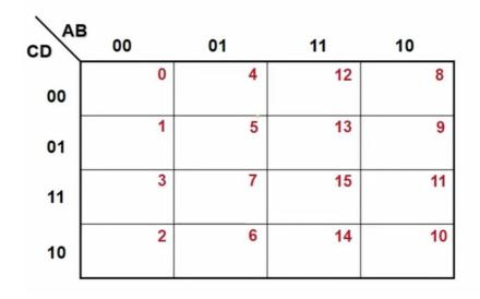
$\underline{\textit{Example:}}$  Using k-map to derive the minimal SOP for the output F(A,B,C,D) of the given truth table:
