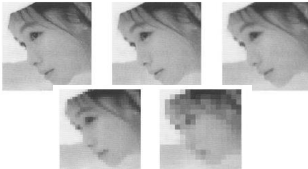
Figure : Images sampled at 256 \times 256 , 128 \times 128 , 64 \times 64 , 32 \times 32 , and 16 \times 16 rectangular sampling grids.
