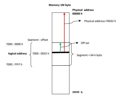
After working through some examples, this will become much clearer to understand: The physical or Absolute address for the Segment:Offset pair, F000:FFFD can be computed by inserting a zero at the end of the Segment value ( which is the same as multiplying by 10 h ) and then adding the Offset value:
