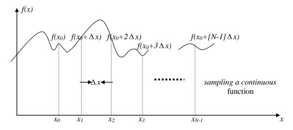
Where x now assumes the discrete values 0,1,2, ...., N-1. In other words the sequence  $\{f(0), f(1), f(2), \dots, f(N-1)\}$  will be used to denote any N uniformly spaced samples from a corresponding continuous function. The discrete fourier transform pair that applies to sampled functions is given by:
