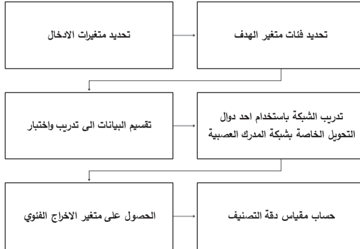
Figure 4: General structure of the perceptron neural network algorithm
