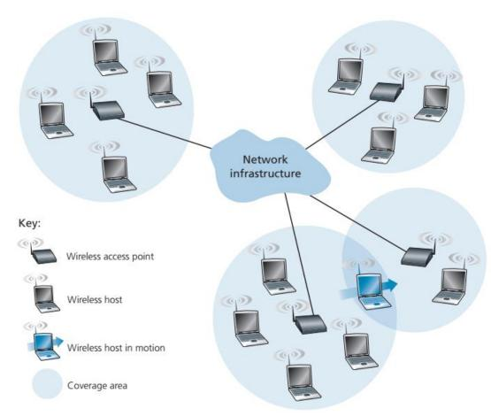
The base station is connected to the larger network (e.g., the Internet, corporate or home network), thus functioning as a link-layer relay between the wireless host and the rest of the world with which the host communicates.
