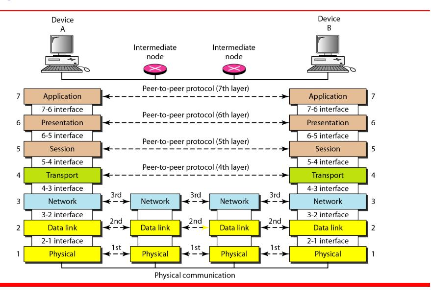
Figure 2.4 An exchange using the OSI model
