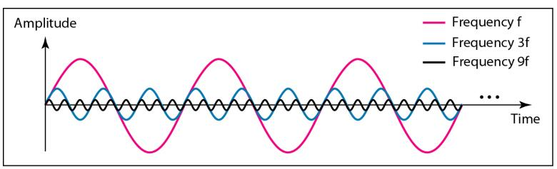
a. Time-domain decomposition of a composite signal
