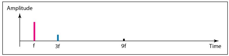
b. Frequency-domain decomposition of the composite signal
