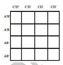
• There are 16 possible min terms in case of a 4-variable Boolean function. The general representation of min-terms using 4 variables is shown below.
