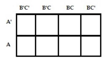
• For a 3-variable Boolean function, there is a possibility of 8 output min terms. The general representation of all the min terms using 3-variables is shown below.
