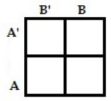
• The possible min terms with 2 variables (AandB) are  $A.B, A.\overline{B}, \overline{A}.B$  and  $\overline{A}.\overline{B}$ . The conjunctions of the variables (A, B) and  $(\overline{A}, B)$  are represented in the cells of the top row and  $(A, \overline{B})$  and  $(\overline{A}, \overline{B})$  in cells of the bottom row. The following table shows the positions of all the possible outputs of 2-variable Boolean function on a K-map.
