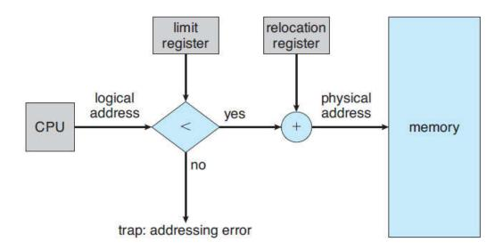
Hardware Support for Relocation and Limit Registers
