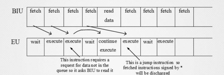
There are three conditions that will cause the BIU and EU to enter a "wait" mode. The first occurs when an instruction requires access to a memory location not in the queue. The BIU must suspend fetching instructions and output the address of this memory location. After waiting for the memory access, the EU can resume executing instruction codes from the queue (and the BIU can resume filling the queue).
