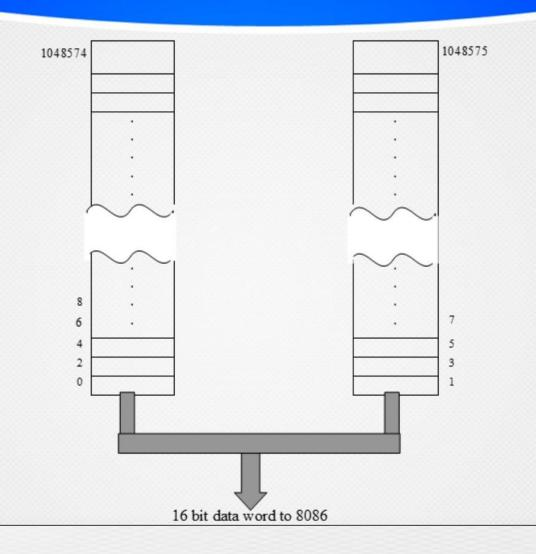
That was for 8086. The 8088 with its 8-bit data bus interfaces to the 1MByte of memory as a single bank. Always when it is necessary to access a word (odd or even) two memory (read or write) cycles are performed, fortunately, for the programmer except for the slightly slower performance of the 8088, there is no difference between the two processors.
