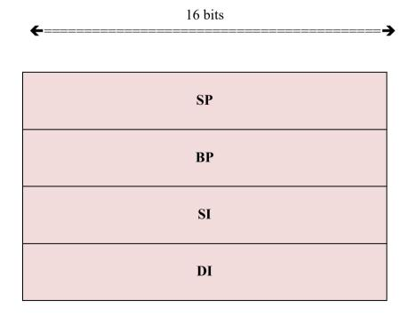
SP: Stack pointer BP: Base pointer SI: Source index DI: Destination index
