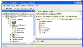
A Graphical User Interface to the database used for configuration and management of the database
