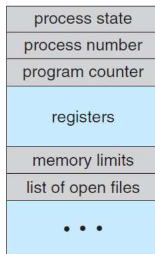
Figure 3: Process Control Block(PCB)
