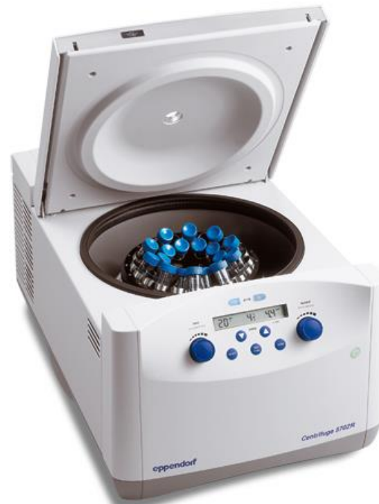
Figure 2: Harvesting bacteria by centrifugation
