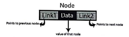
Here, 'link1' field is used to store the address of the previous node in the sequence, 'link2' field is used to store the address of the next node in the sequence and 'data' field is used to store the actual value of that node.
