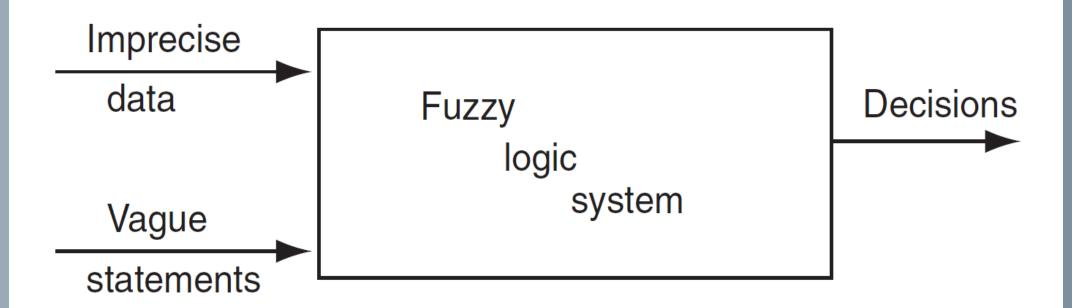
Fig(1): A fuzzy logic system which accepts imprecise data and vague statements such as low, medium, high and provides decisions.
