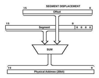
registers are required both to store **segment base address** as well as **offset address**. This makes the internal circuitry easier to build as it removes the requirement for **20 bits** register in case the **linear addressing method** is used.
