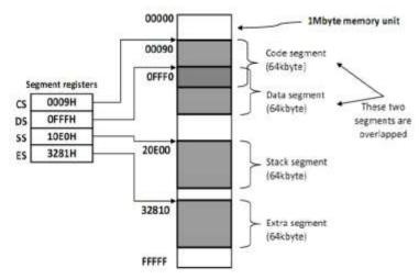
We note here that code segment and data segment are overlapped while other segments are disjointed.
