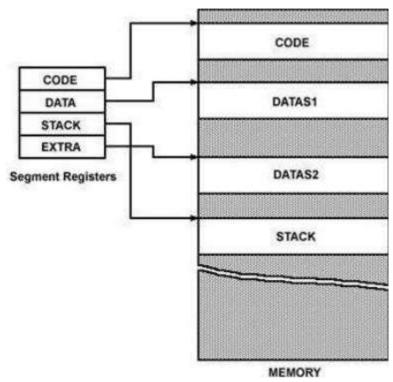
Actually, the 1M bytes of memory are partitioned into 64K byte (65,536) segments. The 8086 microprocessor allow four memory segments.
