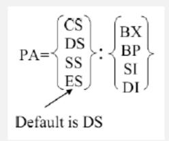
• The [BX], [SI], and [DI] modes use the DS segment by default. The [BP] addressing mode uses the stack segment (SS) by default. You can use the segment override prefix symbols if you wish to access data in different segments.
