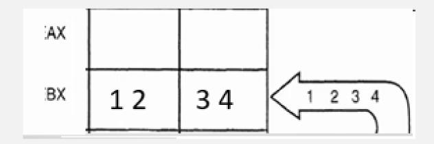
In this mode, the operand is specified in the instruction itself. An immediate mode instruction has an operand field rather than the address field.
