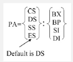
• The [BX], [SI], and [DI] modes use the DS segment by default. The [BP] addressing mode uses the stack segment (SS) by default. You can use the segment override prefix symbols if you wish to access data in different segments.
