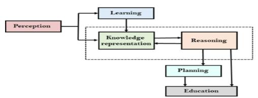
The above diagram is showing how an AI system can interact with the real world and what components help it to show intelligence. AI system has Perception component by which it retrieves information from its environment. It can be visual, audio or another form of sensory
