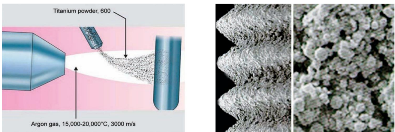
Fig.22: Magnified view of TPS surface (Hadzik, J.; et al 2023).
