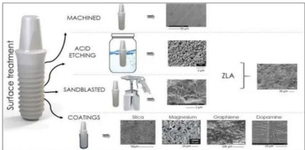
(Fig:18. Various surface modifications of zirconia implants) (Stübinger S.et al.,2008)
