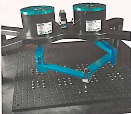
Figure (1):- Five-Bar Parallel Robot With Large Workspace from https://www.researchgate.net/
