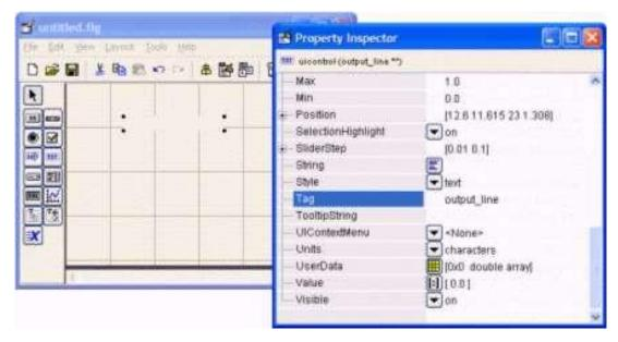
Then, drag-and-drop a 'push button' onto your interface. Modify its 'String' property to read 'Launch Message'. Let its 'Tag' property intact. You could change this tag... it's the name or identifier of the object as it's going to be recognized in the rest of the code.
