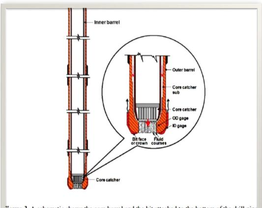
Figure 3. A schematic shows the core barrel and the bit attached to the bottom of the drill pipe
