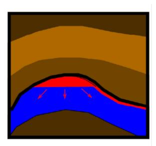
The reservoir is initially strongly water-wet (left). However, once oil migrates into the reservoir, oil displaces water, ageing takes place and the reservoir becomes more oil-wet or mixed-wet (right).
