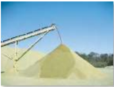
Gravel falling off the end of this conveyor belt follows a path that can be predicted using the equations of constant acceleration. In this way the location of the accumulated pile can be determined. Rectangular coordinates are used for the analysis since the acceleration is only in the vertical direction. (© R.C. Hibbeler)
