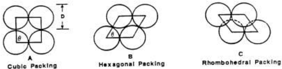
Fig. (4.3): Effect of packing on porosity of uniform spheres.
