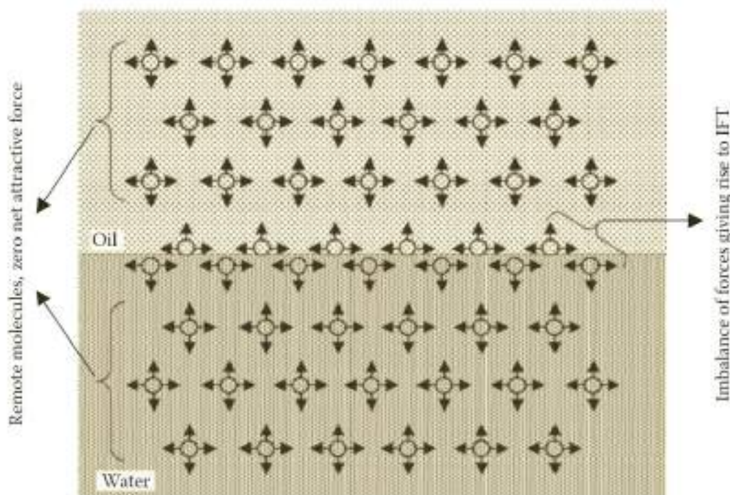
Fig. (4.21): The concept of interfacial tension (IFT) between two immiscible liquids.
