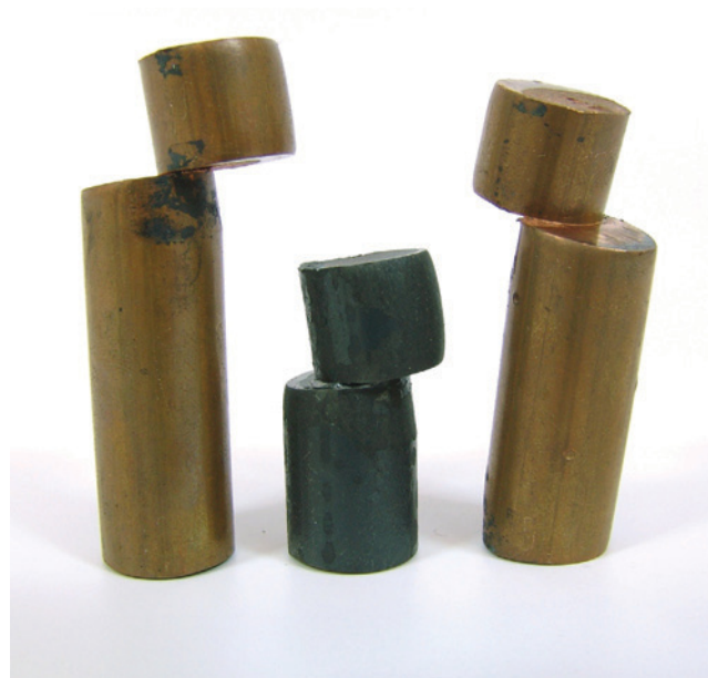
FIGURE 1.3 Single shear failure in pin specimens.
