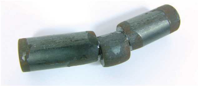
FIGURE 1.4 Double shear failure in a pin specimen.
