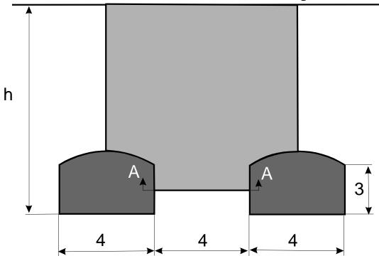
The job is to find the appropriate depth within this range. This is an example for pillar design. The loading condition is determined by assuming that the weight of the overlying rock mass, as shown in Figure 1, is distributed evenly across the width of the pillar at AA (this is not quite true, the stresses are usually higher at the tunnel perimeter than at the center, but the high safety factor should take care of this). You follow this procedure now:
