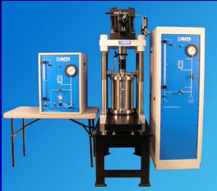
Triaxial rock testing system
