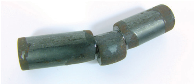
FIGURE 1.4 Double shear failure in a pin specimen.
