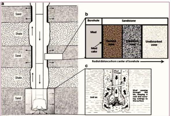
➤ The flushed zone ( $\mathbf{R}_{xo}$ ): a zone occurs *close to the borehole* where the mud filtrate has almost completely flushed out the formation's hydrocarbons and/or water.
