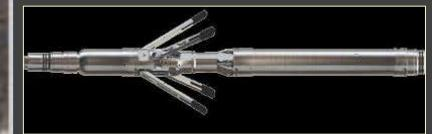
**Mechanical Caliper Log**
